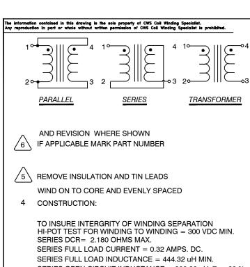
TO INSURE INTERGRITY OF WINDING SEPARATION HI-POT TEST FOR WINDING TO WINDING = 300 VDC MIN. SERIES DCR= 2.180 OHMS MAX. SERIES FULL LOAD CURRENT = 0.32 AMPS. DC. SERIES FULL LOAD INDUCTANCE = 444.32 uH MIN. SERIES OPEN CIRCUIT INDUCTANCE = 802.82 uH @  $\pm$  20 % PARALLEL DCR= 0.545 OHMS MAX. PARALLEL FULL LOAD CURRENT = 0.64 AMPS. DC. PARALLEL FULL LOAD INDUCTANCE = 111.08 uH MIN. PARALLEL OPEN CIRCUIT INDUCTANCE = 200.70 uH @  $\pm$  20 %
